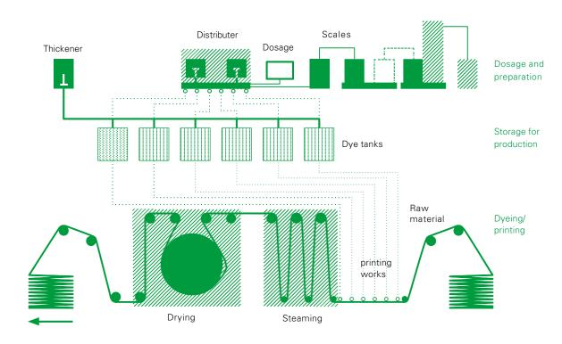
DYE DOSAGE AND BATCH PREPARATION STATION
